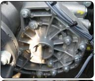
1) Remove the gearbox cover and make sure that the parts belonging to the oil lube pump are well located in their seats.
